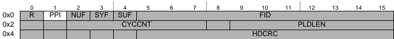
Figure 22-111. Frame Header Structure (Transmit Message Buffer for Key Slot)
