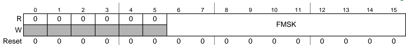
Figure 22-36. Sync Frame ID Acceptance Filter Mask Register (SFIDAFMR)
